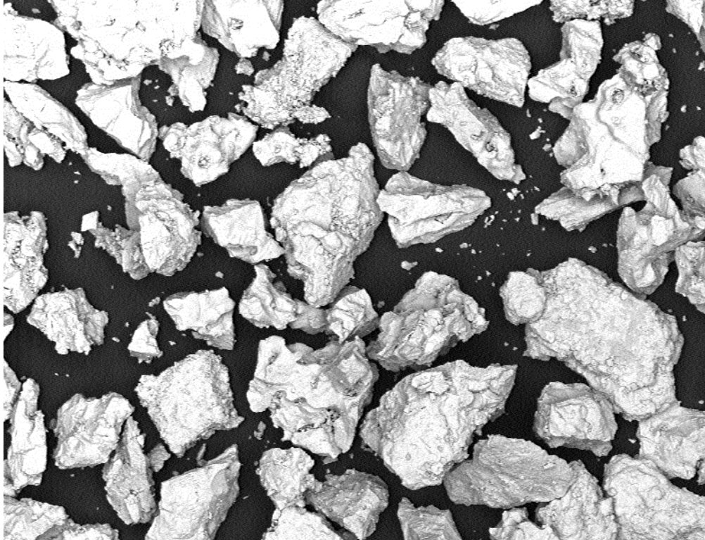
Figure 1: Typical Powder Morphology (SEM 200X)
