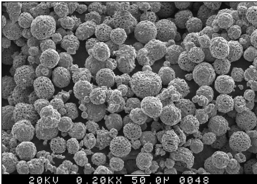
Figure 1: Typical Powder Morphology (SEM 200X)
