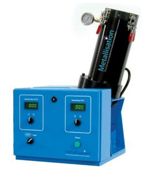
The design of the Metallisation 2007MF-PF powder feeder produces a consistent, repeatable and non-pulsing flow of powder to the plasma pistol. This design of feeder ensures flowability of powders over a wide range of particle sizes.
