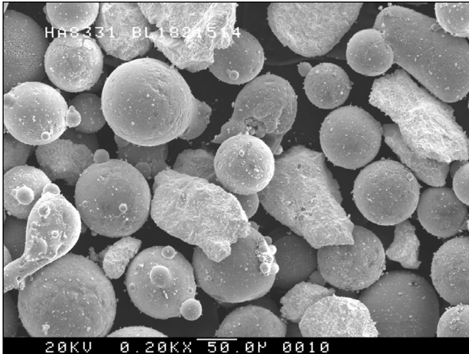
Figure 1: Typical Powder Morphology (SEM 200X)
